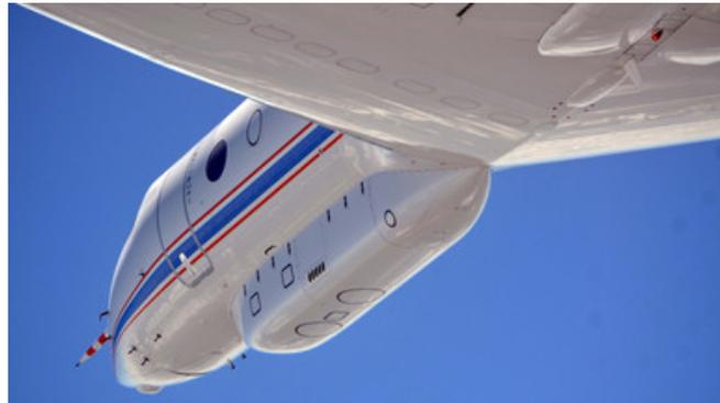
Fig. 2: "Belly Pod" underneath the hull of HALO. It contains radiometers, a radar and a laser for measuring profiles during the flights. (Source: DLR)
