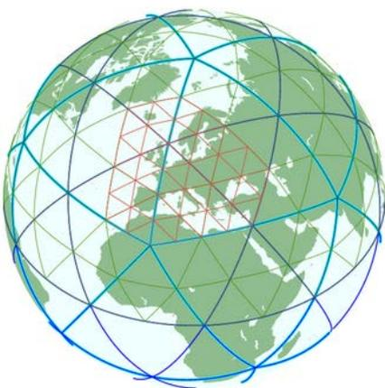
*Fig. 1: Example of a twofold refined regional ICON grid. The light blue grid shows the icosahedron defined base grid with 20 triangular faces, 30 edges and 12 vertices. The dark blue grid was created by a first refinement, in which the edge centers form new vertices. The additional grid refinement was only carried out for the northern hemisphere, depicted by the green grid. The red grid shows another refinement step in the region over Europe.*
