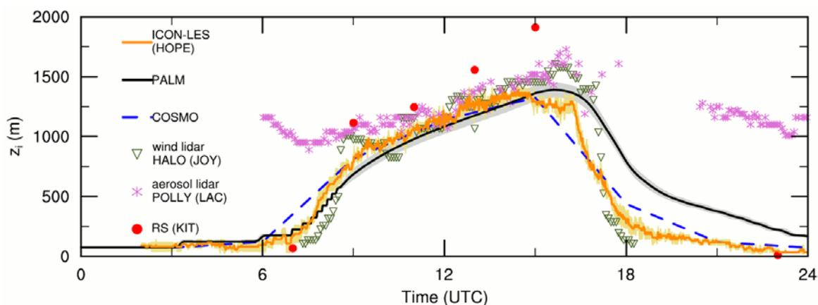
Fig. 4: Temporal progression of the boundary layer depth on 24 April 2013 in lidar and radiosonde measurements and in the Germany-wide ICON simulations (orange). The boundary layer height is shown additionally in the weather forecast model COSMO-DE (blue) and in an idealized simulation with PALM in a smaller area at a resolution of 50 m.
