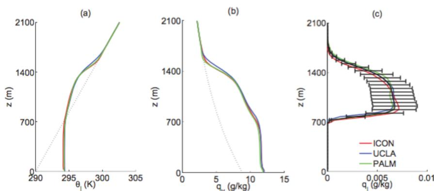
*Fig. 2: Mean vertical profiles of (a) wet-potential temperature  $\vartheta_w$ , (b) the specific humidity  $q_w$ , (c) the cloud liquid water content  $q_l$  in ICON (red) and the two LES models UCLA (blue) and PALM (green). An uncertainty range for this experiment was shown by Siebesma et al. for the cloud liquid water area in a previous model comparison [3].*
