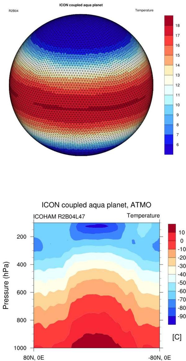
Figure 3. On top: sea surface temperature in °C. Snapshot after two years of simulation time. At bottom (left and right): temperature in °C in the atmosphere and ocean in a north-south cross section at 0° longitude
